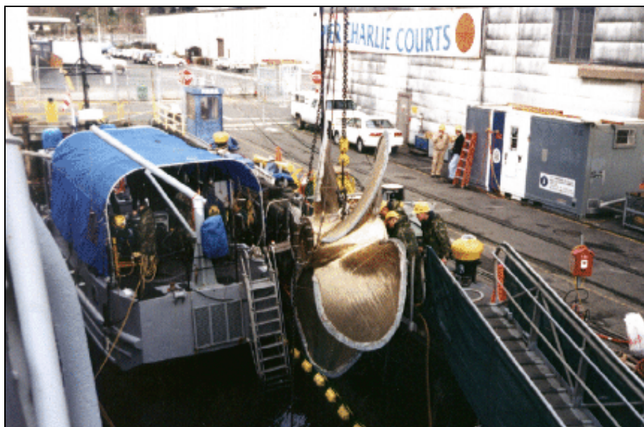
Divers installing gland ring studs on the new propeller hub.
