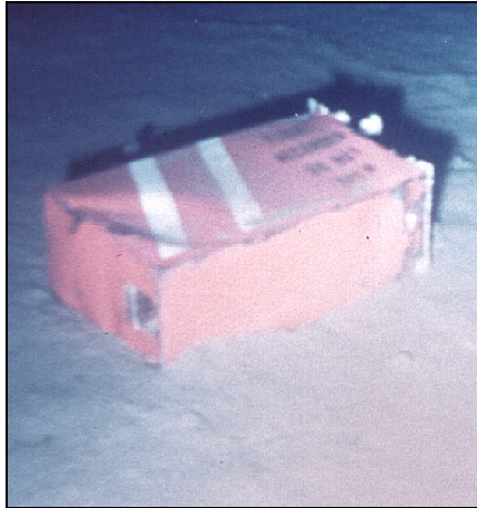
The flight data recorder lies on the sandy bottom of the Atlantic, 7,200 feet from the surface.
