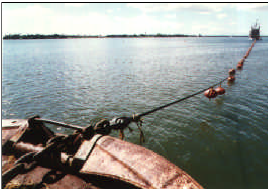
(Salvage training) Coming up to strain. Normally a pull of about 60,000 lbs. is required to free the training hulk Tunica .
